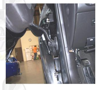
**9)** Cut the inner lip of your fender to make room for the new Vertical Doors hinge. Note: After you have cut the fender use a sander or grinder and make sure the surface is completely flat.
