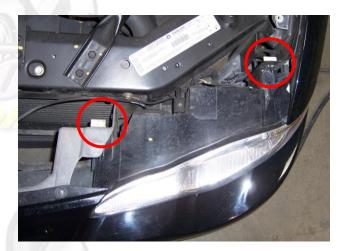
Remove all Phillip's screws and plastic fasteners from the wheel well.
