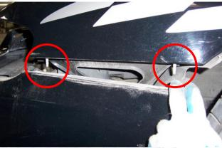
Now pull on the bumper to gain access to (1) 10mm bolts securing the fender to the body.
