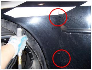
Remove (2) 10mm bolts located at the bottom of the door, securing the fender to the body.
